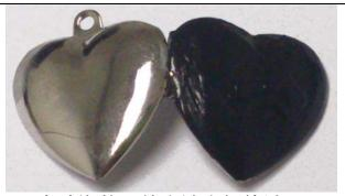
在清潔的工件上塗上絕緣油, Apply plating resist on cleaned goods.
